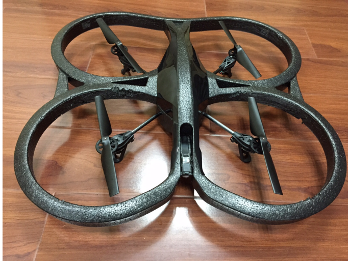
Figure 1: The AR.Drone 2.0 in our project, with the front camera modified to toward down
