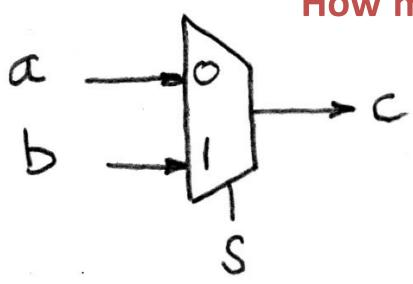
$$c = \overline{s}a\overline{b} + \overline{s}ab + s\overline{a}b + sab$$
