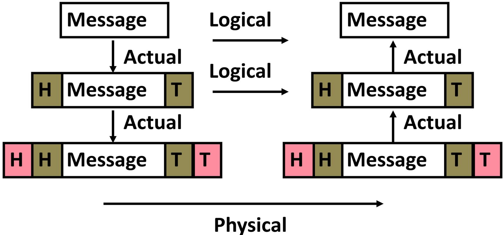
*Each lower level of stack “encapsulates” information from layer above by adding header and trailer.*
