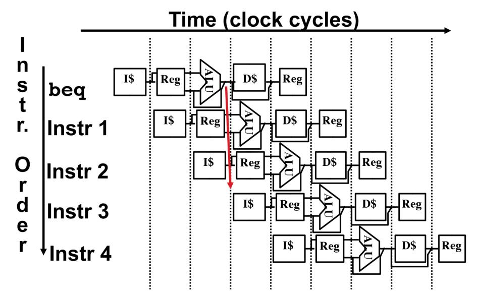
We found that the instruction fetch and memory stages are the critical path of our 5-stage pipelined MIPS CPU. Therefore, we changed the IF and MEM stages to take **two** cycles while increasing the clock rate. You can assume that the register file is written at the falling edge of the clock.
