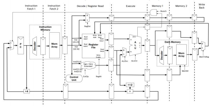
Assume that no pipelining optimizations have been made, and that branch comparisons are made by the ALU. Here's how our pipeline looks when executing two add instructions:
