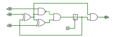
(b) What is the critical path delay, and what is the maximum clock frequency at which the circuit will operate correctly?
