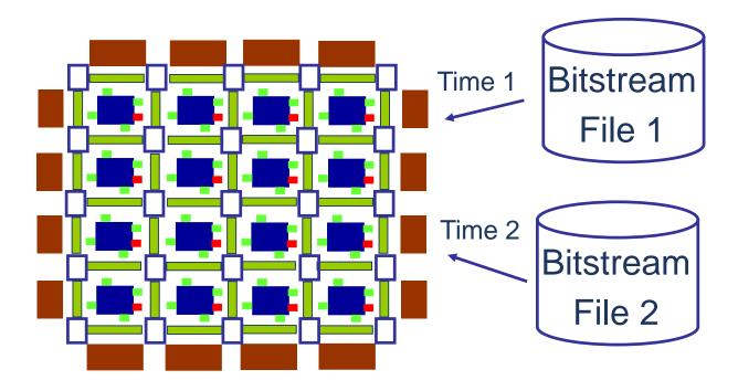
All the programming information for the three FPGA components is stored in a configuration file. The configuration file for a FPGA is often called a *bitstream* compared to a binary executable for a processor. Once a bitstream for a digital logic design is downloaded to a FPGA, the FPGA is programmed to implement the design. By providing different bitstreams, a single FPGA can be reprogrammed to implement different designs at different times.
