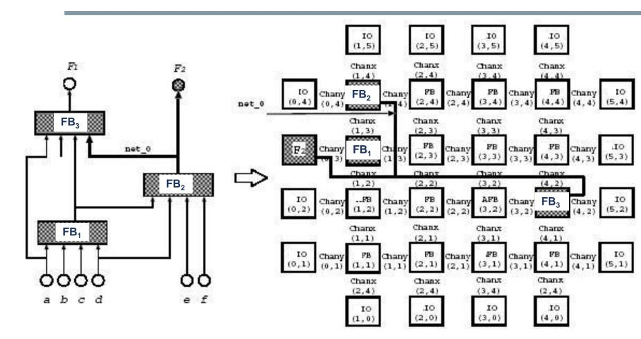
The placement step finds physical locations for functional blocks, while the routing step finds physical routes for logic connections.
