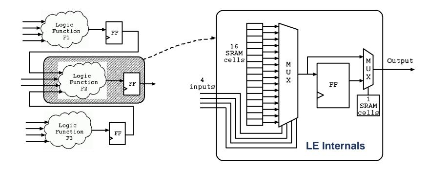
The LE consists of a 16 SRAM cell Look-Up Table (LUT), and a flip flop (FF). The 16 SRAM cells LUT stores the truth table of any 4-input logic function, thus it can implement any 4-input logic function. The FF implements the storage element in a sequential circuit.
