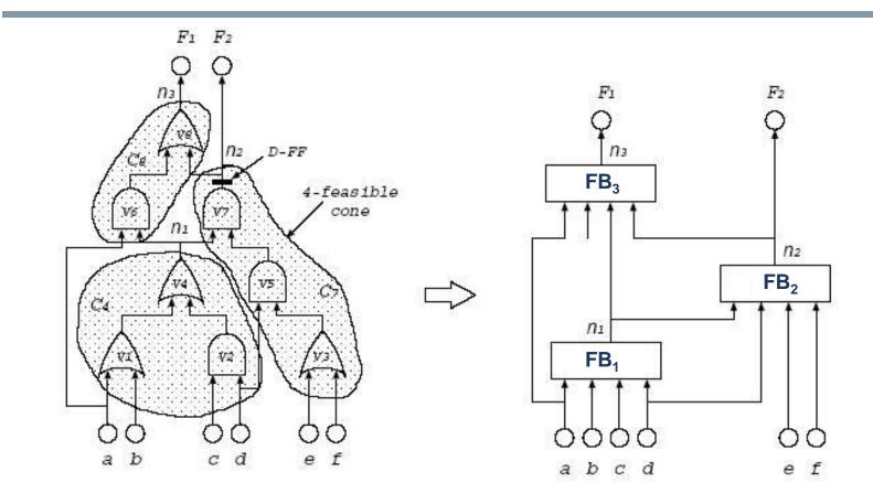
Technology step restructures the primitive logic gates, generated from the logic optimization step, into sets of 4-input functional blocks (We assume one functional block contains only one logic element in this example).
