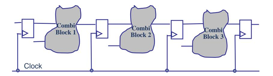
• Clocks are used to synchronize the start of computations in all combinational blocks.
