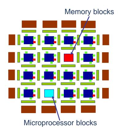
• Besides the LEs present in previous slide, some functional blocks in different FPGAs have architecture specific features to improve the performance when implementing arithmetic functions.
