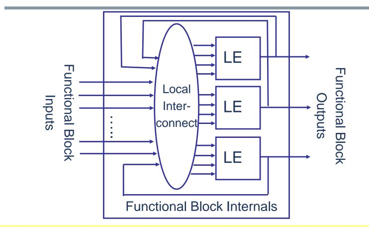
FPGAs use the Look-Up Table (LUT) type of functional block. Such a functional block is normally made of one or several logic elements (LE). They differentiate from each other mainly in terms of the input size of a LE and the number of LEs in a functional block. State-of-the-art FPGAs normally use 4-input LEs.
