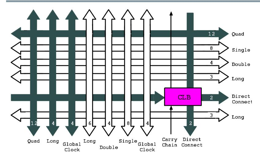
In Xilinx terms, a functional block is called a CLB (Configurable Logic Block).
