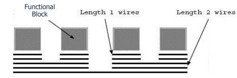
wires Length 4 wires
