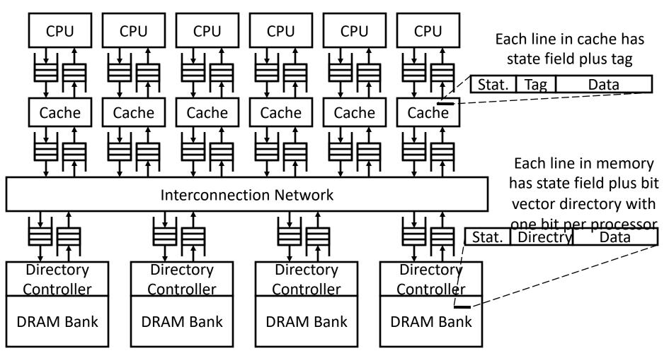
Assumptions: Reliable network, FIFO message delivery between any given source-destination pair
