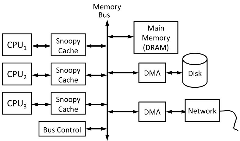
Use snoopy mechanism to keep all processors' view of memory coherent
