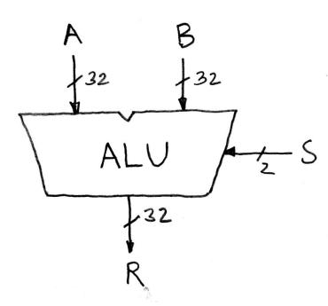
when S=00, R=A+B when S=01, R=A-B when S=10, R=A AND B when S=11, R=A OR B
