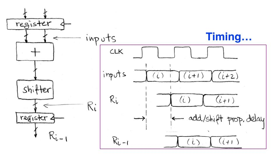
Note: delay of 1 clock cycle from input to output. Clock period limited by propagation delay of adder/shifter.
