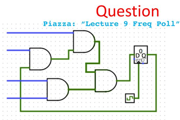
Clock->Q 1ns Setup 1ns Hold 1ns AND delay 1ns
