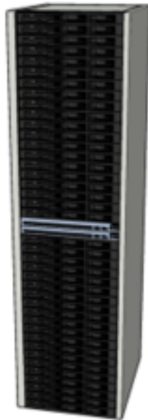
7 foot Rack: servers + Ethernet local area network switch in middle (“rack switch”)
