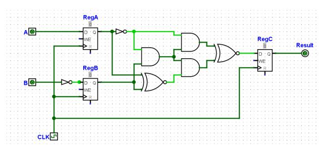
(a) What is the minimum acceptable clock cycle time for this circuit, and the clock frequency this corresponds to?
