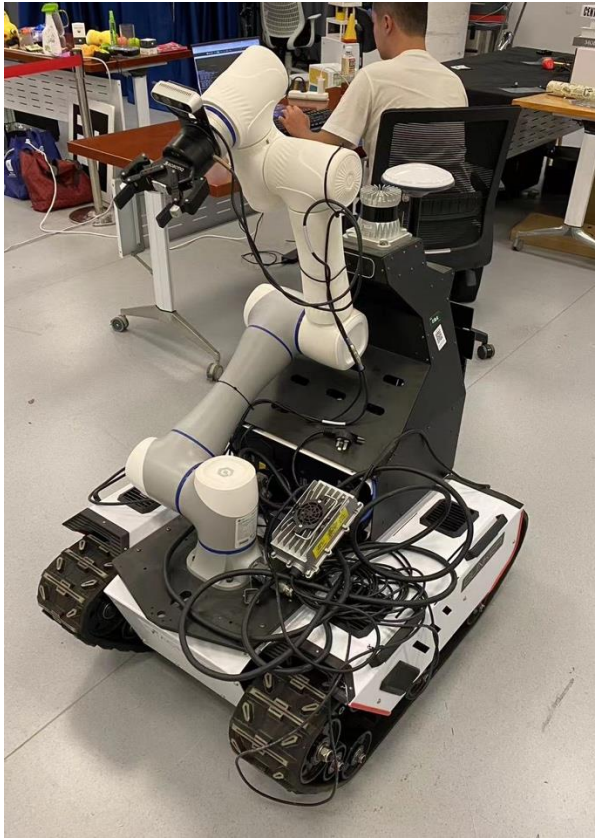
Agile X Bunker Tracked Mobile Robot with Dobot Arm
