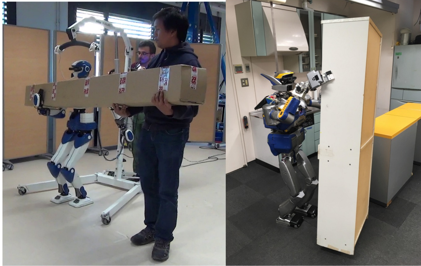
Fig. 3: (left) HRP-4 holding a large box with a human while walking (Agravante et al. (2019)) (right) HRP-2 pivoting a furniture (Murooka et al. (2017)).
