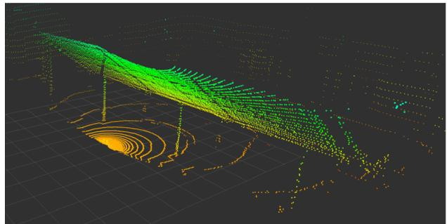
Figure 2. Original point cloud with solar panel and rods
