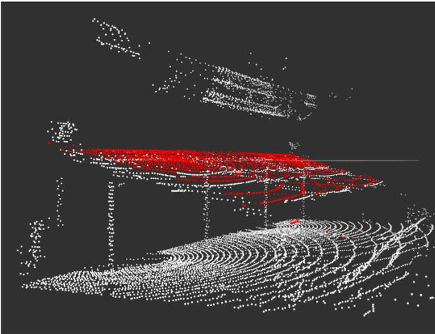
Figure 4. Point cloud of detected solar panel
