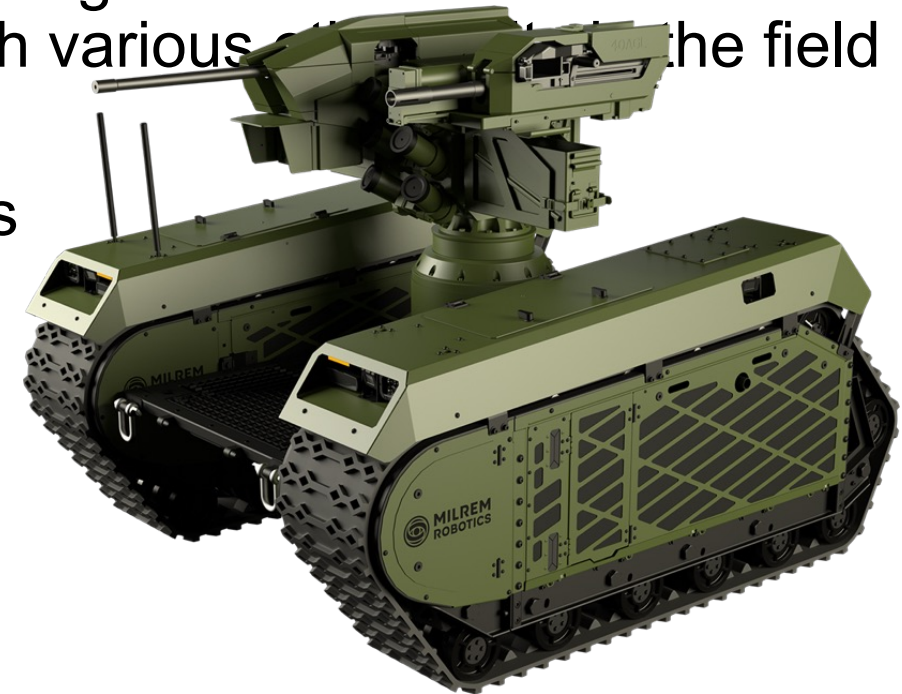
THeMIS robot from the Estonia company MILREM Robotics. The 2t semi-autonomous robot can drive with a speed of up to 20km/h.
