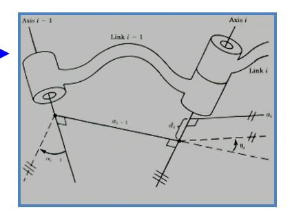
For Prismatic Joints: a,  $\alpha$ , and  $\theta$ . are all fixed, then " $d_i$ " is the.
