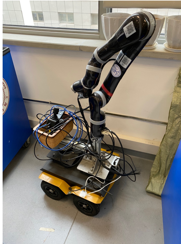
Jackal Mobile Platform with Kinova Robot Arm
