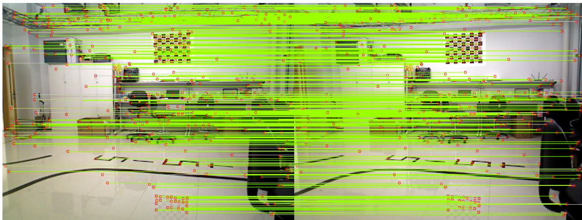
Figure 4-2 Extract and match the features between two images (Same position)
