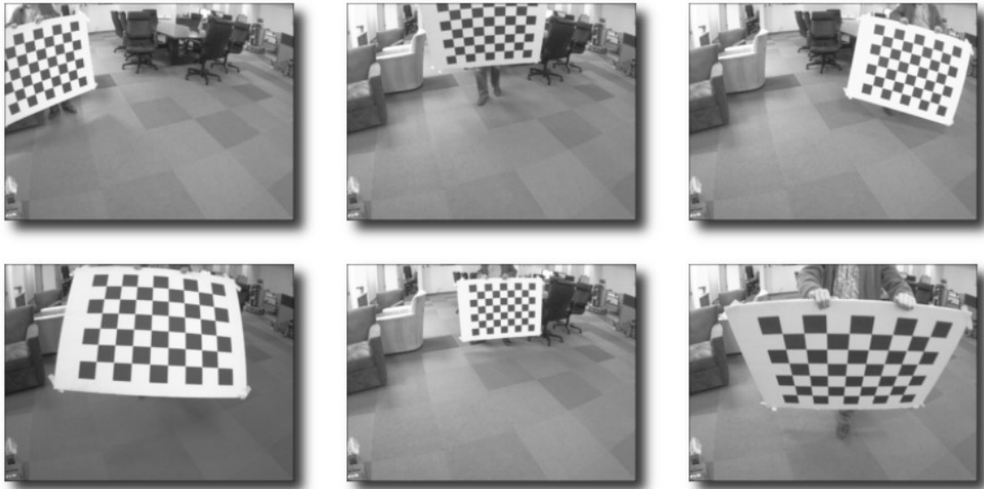
Figure 2-11 Checkerboard lies on the camera's left and right, top and bottom of field of view(the 1-3th picture); toward/away and tilt from the camera(the 4-5th picture); checkerboard filling the whole field of view(the 6th picture) [43]
