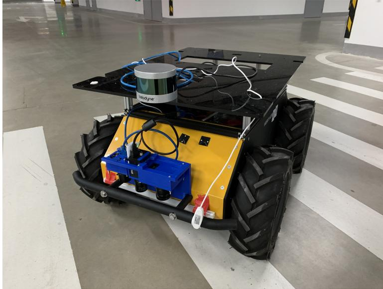
Figure 1: The husky robot in a garage, with downward-facing sensors, a bumper and assisted lights in the front, Lidar on the top.
