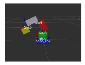
Figure 4. URDF model of the Dobot Magician Arm
