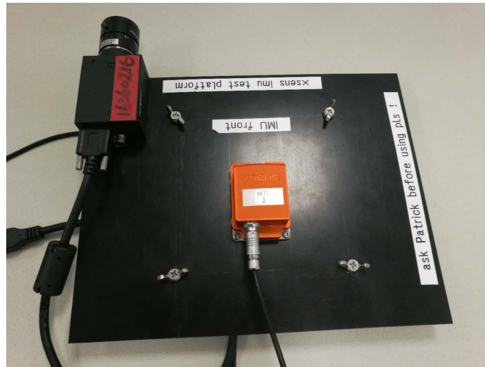
Figure 14: The camera and the IMU we used to calibrate their relationship
