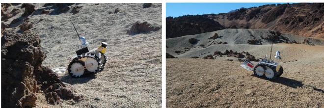
Fig. 3. The two robots of the Jacobs team during the ESA Lunar Robotics Challenge. On the left, the relay robot with a 3D Laser Range Finder to generate models of the environment. On the right, the probe robot to take soil samples in the crater. The photos are taken during the day with good visibility conditions.
