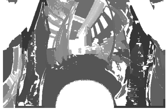
Fig. 4. The 541 \times 361 range-image corresponding to the first scan, with the planar regions identified. This image actually lies on the surface of a sphere, and displaying it as a planar rectangle leads to an obvious distortion.
