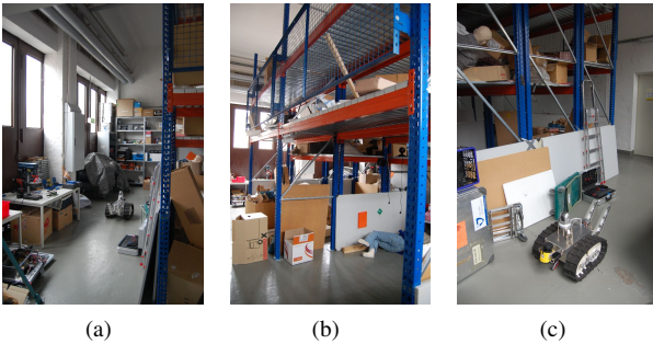
Fig. 3. The robot collecting data in the locomotion test arena in form of a high bay rack
