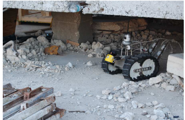
(d) The robot collecting data under the collapsed ceiling of the “ground floor” under the car. The yellow rotating LRF sensor is clearly visible.
