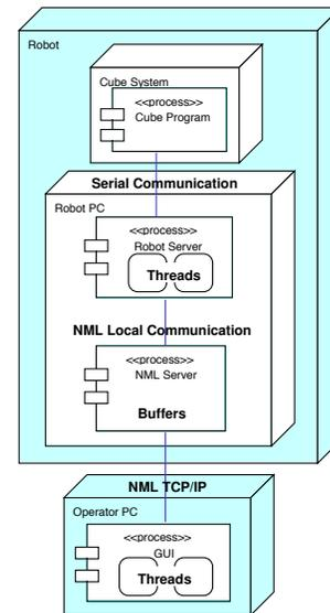
Fig. 5. UML Deployment diagram showing the overall system.
