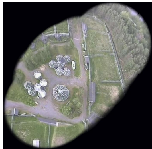
Fig. 2. An example of a photo map of a camp generated during a surveillance mission from 784 video frames in real time.
