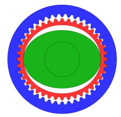
$\label{eq:reduction} \mbox{reduction ratio} = \frac{\mbox{flex spline teeth} - \mbox{circular spline teeth}}{\mbox{flex spline teeth}}$
