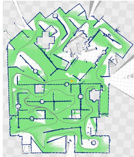
Fig. 3. A very good map created by a human carrying a lightweight robot around. In contrast to Figure 2, the arena is now configured as one big maze for the autonomy challenge. The map is colored after the RoboCup standard, marking white areas as observed but additionally marking areas that were extensively searched for simulated disaster-victims as green. The robot-path, start pose and a 1m grid in the background are also visible.
