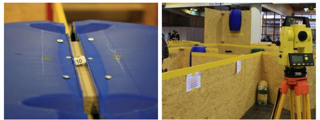
Fig. 4. Left: The middle of a fiducial with marker. Right: A tachymeter set up next to a RoboCupRescue arena to measure the position of the fiducials.
