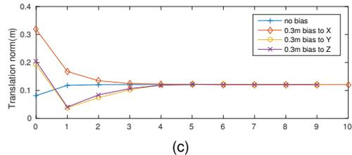
Fig. 5. Gripper-camera experiment. (a) set-up of gripper-camera calibration experiment. (b) reconstruction result. (c) the norm of final translation after biasing the translation estimated by initial hand-eye calibration.
