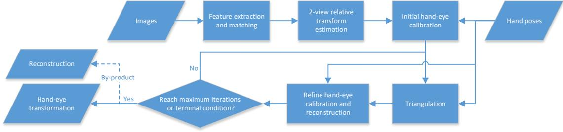
Fig. 2. Block diagram of the proposed hand-eye calibration algorithm.
