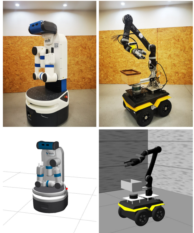
Fig. 2. Mobile Manipulation Systems used in MoManTu: Fetch, real and simulated; Jackal & Kinova, real and simulated.
