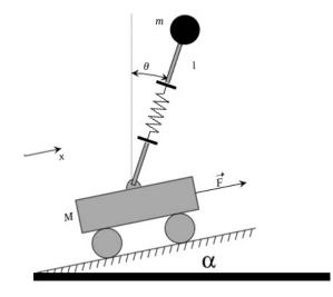
Figure 2: Inverted Spring Pendulum
