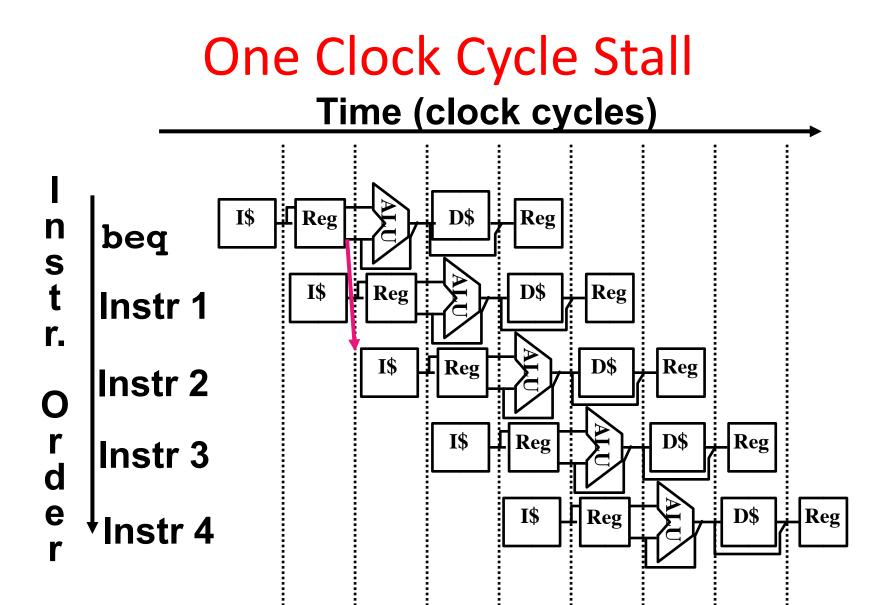
Branch comparator moved to Decode stage.
