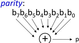
Each word, as it is read from memory is "checked" by finding its parity (including the parity bit).
