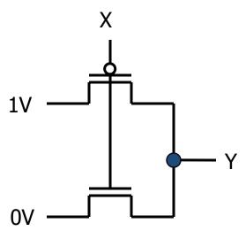
*n-channel transitor* off when voltage at Gate is low on when: voltage(Gate) > voltage (Threshold) what is the relationship between x and y?
