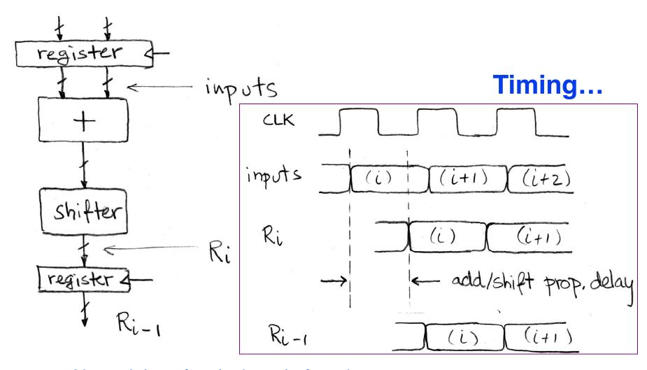
Note: delay of 1 clock cycle from input to output. Clock period limited by propagation delay of adder/shifter. Pipelining to improve performance
