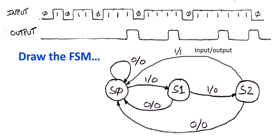
Assume state transitions are controlled by the clock: on each clock cycle the machine checks the inputs and moves to a new state and produces a new output...
