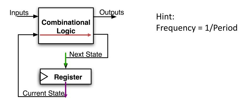
Max Delay = CLK-to-Q Delay + CL Delay + Setup Time
