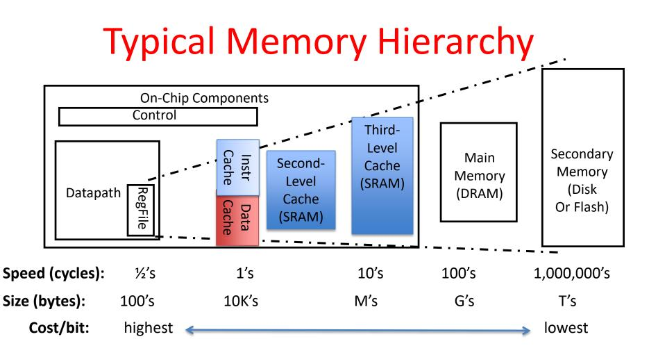
Principle of locality + memory hierarchy presents programmer with ≈ as much memory as is available in the *cheapest* technology at the ≈ speed offered by the *fastest* technology
