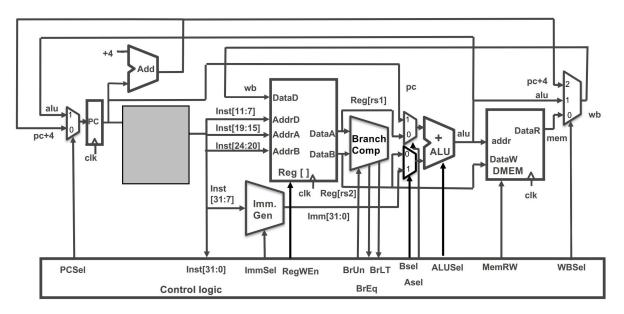
(a) Write down control signals for jal 64. Please use \* to indicate that what this signal is does not matter.
